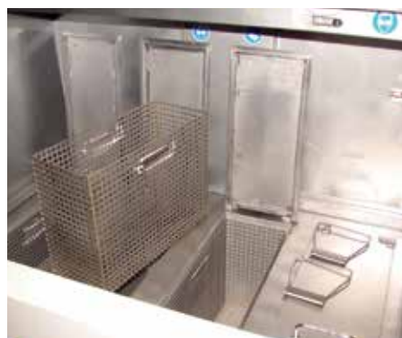
▲ Paint stripping tanks with baskets
