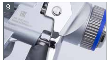
Grease visible part of air piston rod
