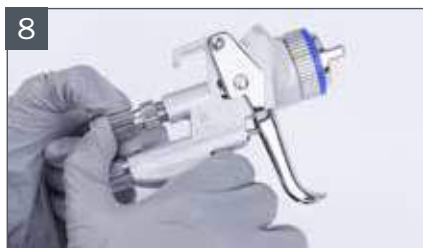
Install material flow control screw
