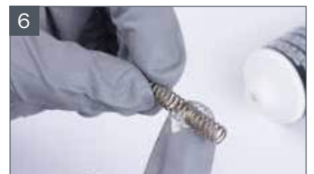
Grease and insert paint needle spring
