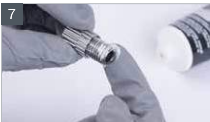
Grease thread of material flow control screw
