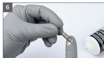
6 Grease and insert paint needle spring
