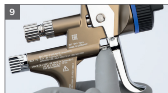
9 Grease visible part of air piston rod
